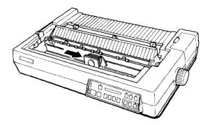
**4.** Turn the ribbon-tightening knob on the ribbon cartridge in the direction of the arrow.
